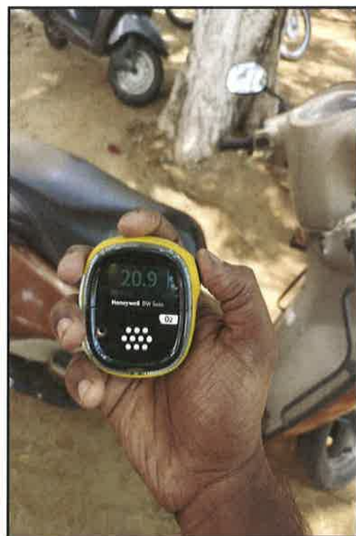
Figure 2. The oxygen concentration in the and O 2 level measured at the Organization using O 2 Meter
